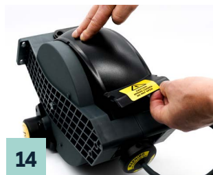
Inserting the middle guide tabs by initially attaching the cover at a slight angle from the side and then final snapping into place.
