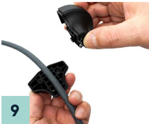
9 Attaching the cable pull stopper to the connection cable, mounting it approximately 1-1.5 meters away from the handheld device.
