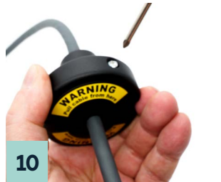
9 Attaching the cable pull stopper to the connection cable, mounting it approximately 1-1.5 meters away from the handheld device.
