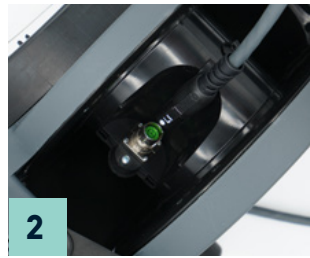
2 Plugging in the cable to the built-in male connector.
