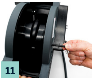
Loosening the nut from the locking pin of the pre-tensioned drum reel.
