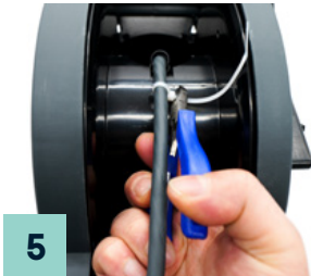
5 Cutting off the excess cable tie.
