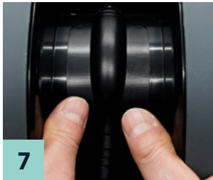
7 Locking the cover by pressing it down.
