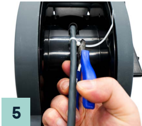
5 Cutting off the excess cable tie.
