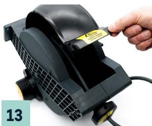
13 Inserting the middle guide tabs by initially attaching the cover at a slight angle from the side and then final snapping into place.
